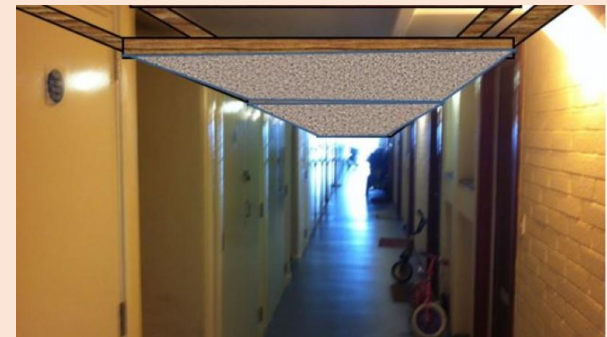
Addition of false ceiling
