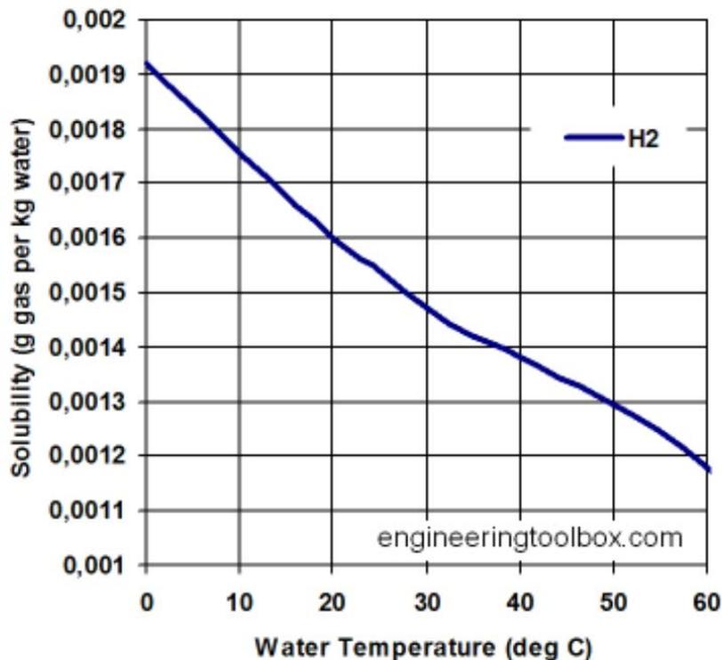
Figure 3. Solubility of H<sub>2</sub> in H<sub>2</sub>O g gas H<sub>2</sub> / kg H<sub>2</sub>O [4]
