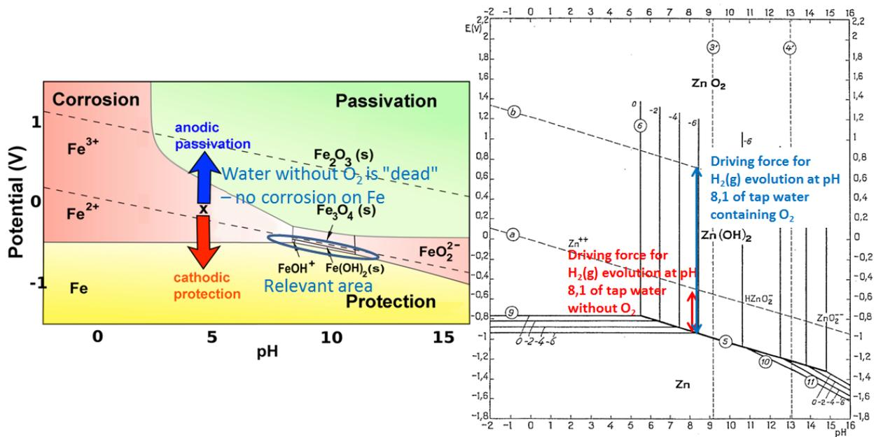
Figure 2. Stability diagrams (Pourbaix) of the iron and zinc chemistry. The thermodynamical driving forces for the hydrogen evolution are seen in the figure [2].
