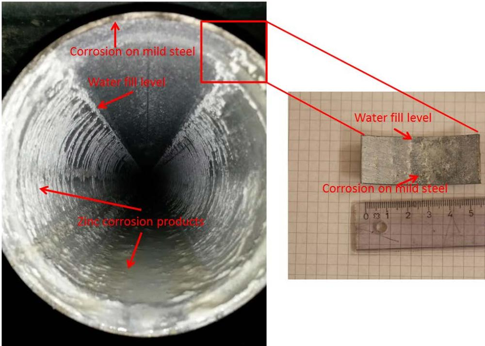
Figure 1. View of the joining area of a galvanized steel pipe with white corrosion products
